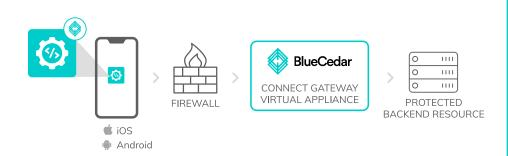
This diagram shows the deployment of the Blue Cedar Connect Gateway as part of Blue Cedar's secure connectivity offering. On the left side of the diagram is a mobile app into which a VPN client has been integrated without coding through the use of the Blue Cedar Accelerator for Secure Edge Connect.
