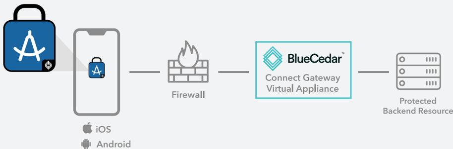
*This diagram shows the deployment of the Blue Cedar Connect Gateway as part of Blue Cedar's secure connectivity offering. On the left side of the diagram is a mobile app into which a VPN client has been integrated without coding through the use of the Blue Cedar Accelerator for Secure Edge Connect.*
