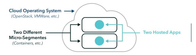
**Figure 3-3.** Containerized Micro-Segmented App Hosting
